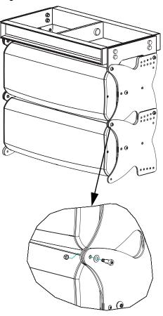
Figure 8:PB2082-i under WL2082-i attached to FB2082-i.
