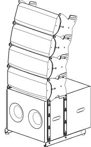
Figure 14: WL2082-i attached to WL115-sw and FB2082-i.
