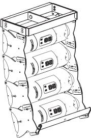
Figure 9: Bolting order for EB2082-i Extension Bar rigging plates.
