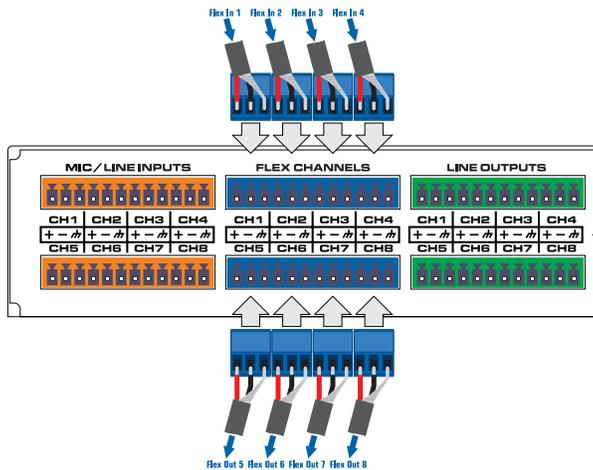
Figure 4. Connecting the Flex inputs and outputs.
