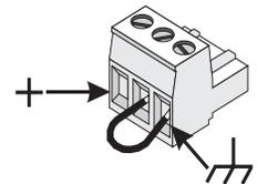
**Omni In connections. Variable input must be 10k ohm variable resistor. Contact closure input can be a switch or relay contacts. These inputs can operate software "devices". Negative (-) terminal is at chassis potential.**
