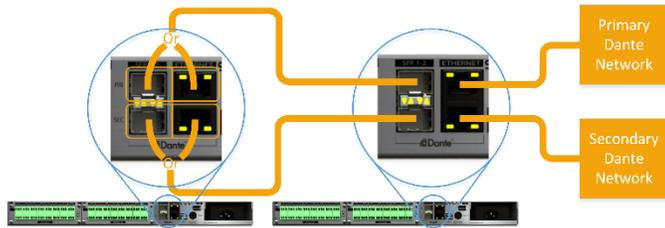
**Figure 5 - "Redundant" mode with daisy chaining**
