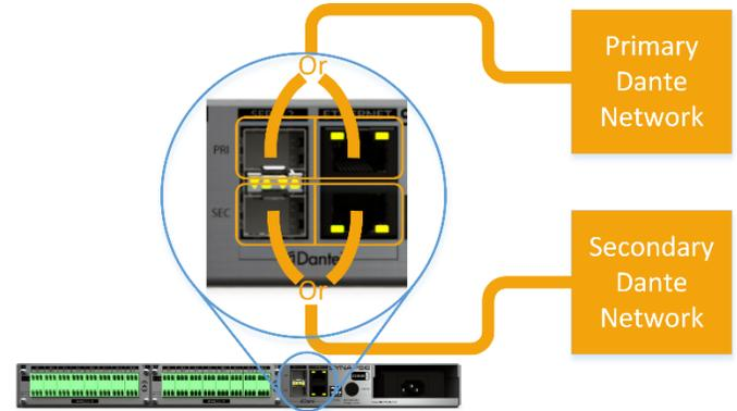
Figure 4 –“Redundant” mode, no daisy chain
