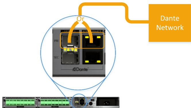
**Figure 6 - "Standalone" connection in “Redundant” mode**
