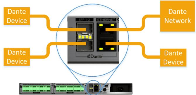
**Figure 7 - "Standalone" connection in "Switched" mode**
