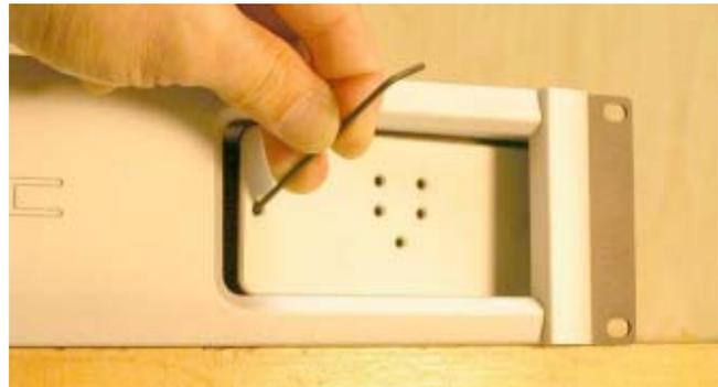
**3-** Once the right side has been withdrawn from its retaining slot, pull the gain control lockout plate out from the front panel recess.
