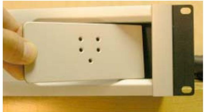
2- While lightly pressing the right side of the cover against the chassis, use the hex key tool (inserted into the plate's screw hole) to slide the cover to the left until the LEDs line up with the cover's holes. Continue to lightly press the cover against the chassis while you insert the cover's retaining screw and secure the screw. Fully tighten the retaining screw.
