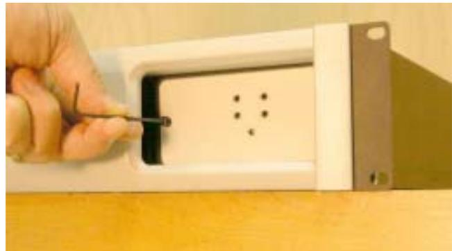
**2-** Insert the end of the hex key tool into the cover's screw hole and pull/swing the plate out as shown.
