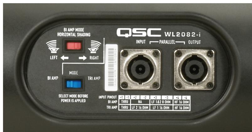
which driver—right or left—to shade. For maintaining optimal stereo imaging with a left and right array arrangement, select the shaded sides so that they are symmetrical—i.e., either all on the outside or all on the inside.
