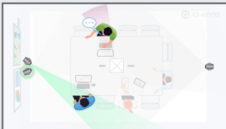
Secondary Camera Rotates to Face Second Talker
